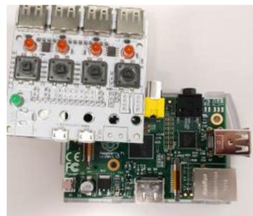
Connect a power such as a mobile battery to this board.
