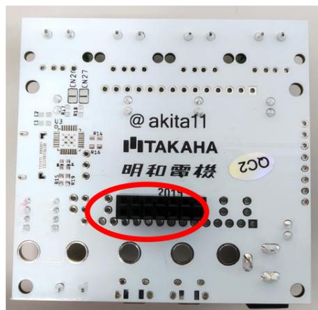
Connect to GPIO connector of Raspberry Pi. See below image.
